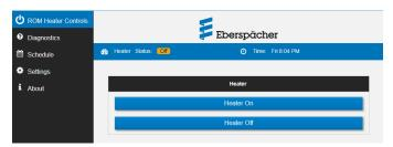
This is where you can control your heater controller device, setup a desired schedule, or see heater diagnostics if your heater isn't working.
